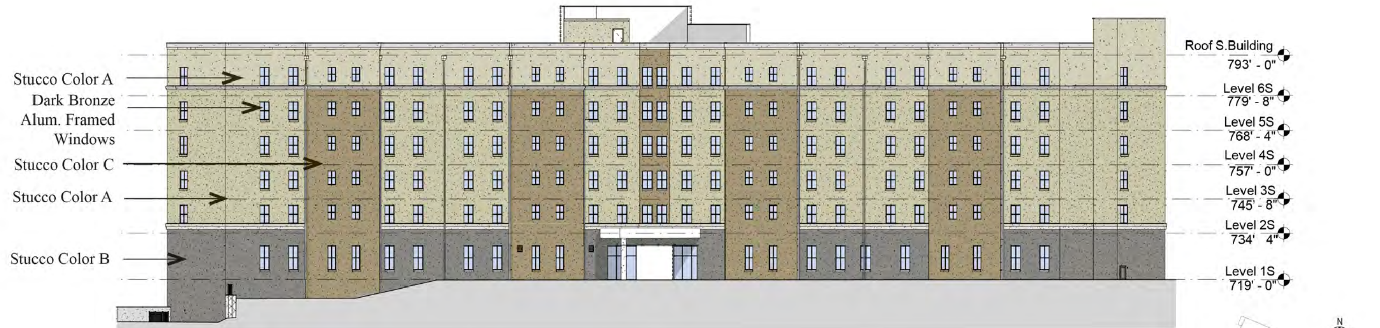
South Building - Northeast Elevation A2.00 1/32" = 1'-0" 0 8' - 0" 16' - 0" 32' - 0" 64' - 0"
