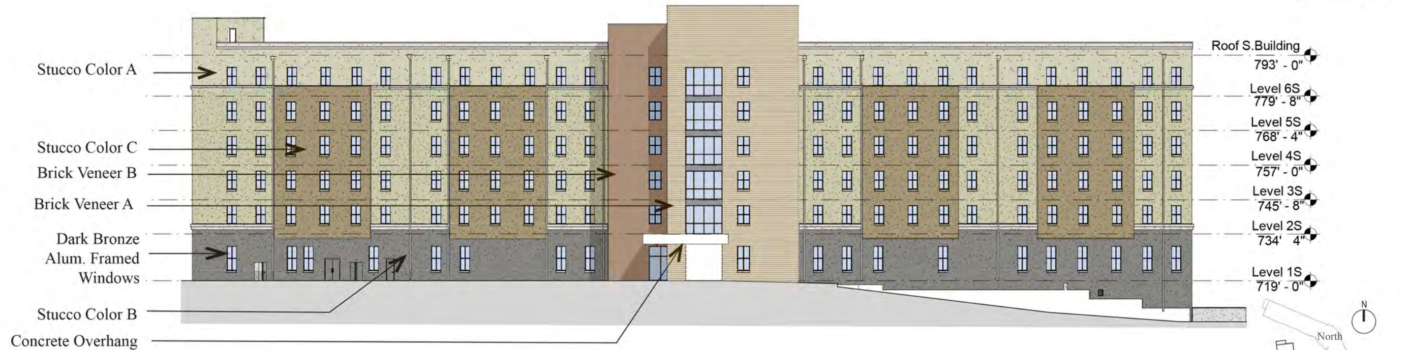
South Building - Southwest Elevation A2.00 1/32" = 1'-0" 0 8' - 0" 16' - 0" 32' - 0" 64' - 0"
